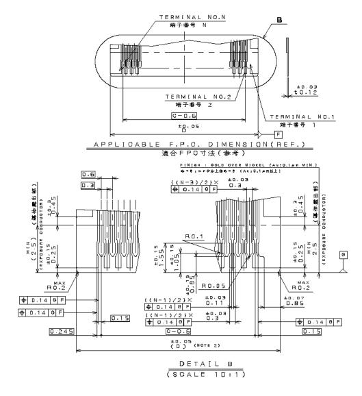
Note 2) To improve reliability of pitch direction positioning accuracy +0.05 -0.01 is recommended for dimension D.
