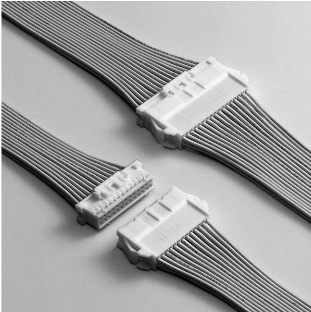
2.5mm (.098") pitch grid (dual in row) wire-to-wire connector that can mate with the socket of XAD connector (board-to-wire type).
