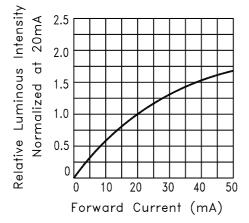
Fig.4 RELATIVE LUMINOUS INTENSITY VS. FORWARD CURRENT
