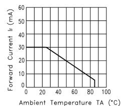
Fig.3 FORWARD CURRENT DERATING CURVE
