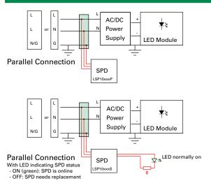
Note: Series module used in parallel connection for indication circuit connection.
