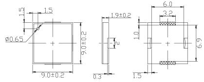
Units do not come with wash label and are not appropriate for aqueous wash. **Packaging:** Parts are supplied on tape-and-reel, 1000 pcs/reel.
