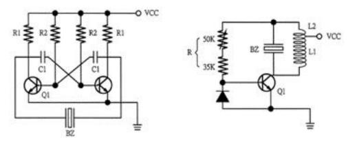
The following three circuits provide a means to drive the electromagnetic transducer buzzer, but they require an input signal to turn the drive circuitry off and on at the appropriate rated buzzer frequency. Care must be taken not to over-voltage the buzzer.
