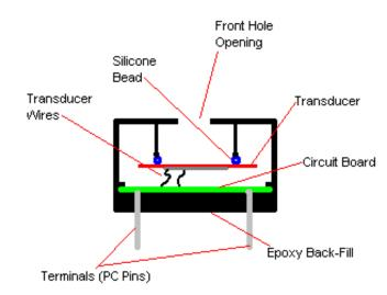
Piezoelectric Audible Signal Basic Construction
