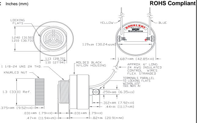
NOTE A: TERMINALS-.032 BRASS TIN PLATED, TAPPED FOR #6-32 SCREW. TWO #6-32 NICKEL PLATED BRASS SCREWS INCLUDED. WILL ACCEPT 1/4" QUICK CONNECT. NOTE B: MOUNTING- REMOVE BLACK PLASTIC NUT AND INSERT THREADED FRONT THROUGH 1.25" HOLE PUNCHED IN PANEL, IF ORIENTATION IS NEEDED, NOTE LOCKING FLATS ON DRAWING. SCREW NUT BACK ON. DO NOT OVERTIGHTEN.
