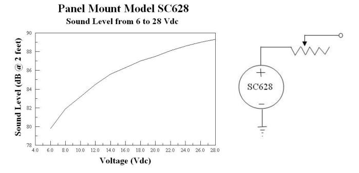
It was verified that the circuitry of model SC628R is not affected by a potentiometer, so data was gathered to find the value of a potentiometer that gives the greatest range of sound change.
