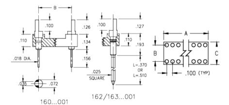
Description: DIP Header Slotted Header Solder Tail Open Frame Through Hole Plating Code: 10
