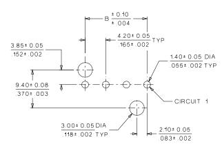
PCB LAYOUT: COMPONENT SIDE RECOMMENDED PCB THICKNESS:  $\frac{1.78}{0.70}$  MAX
