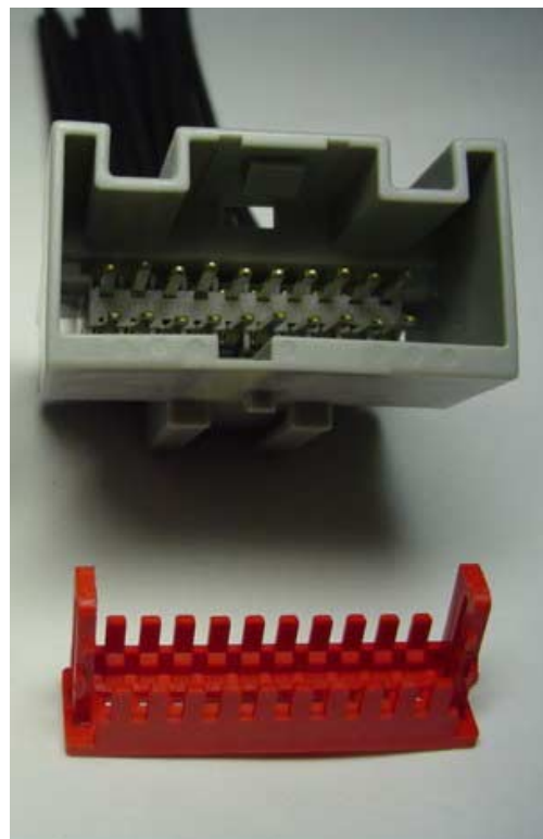
Un-damaged TPA after removal
