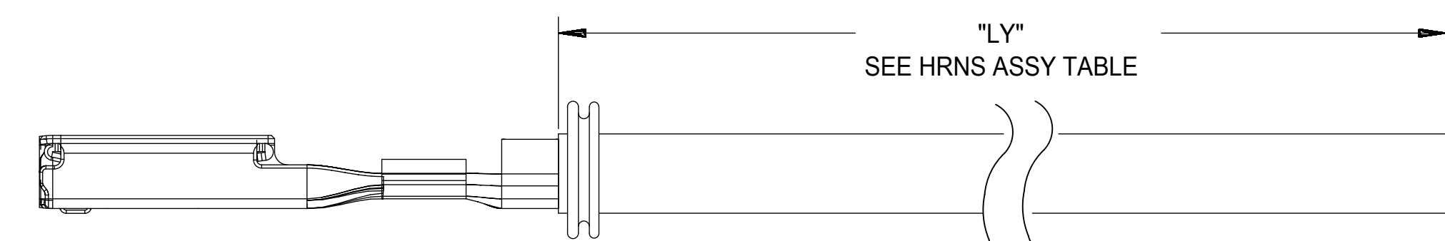
2.8mm YESC SEALED FEMALE PIGTAIL ASSY MATERIAL #: SEE HRNS ASSY TABLE
