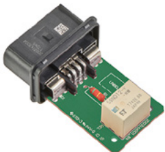
1 Relay, Supporting Electronics 200316-1101 (Application Example: Cooling Fan)
