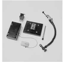
This application tooling was designed specifically to press in the Mini-Fit, CP connector series 43879
