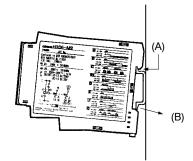
When removing the H3DE, pull out portion (C) with a flat-blade screwdriver and remove the Timer from the mounting track.
