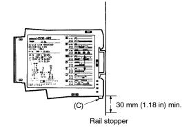
The H3DE can be mounted or removed easily if a distance of 30 mm (1.18 in) or more is kept between the H3DE and the top surface of other equipment located below the H3DE.
