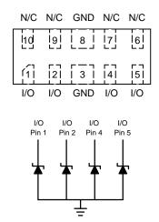
Pins 3, 8 Note: Common GND – Only Minimum of 1 GND connection required
