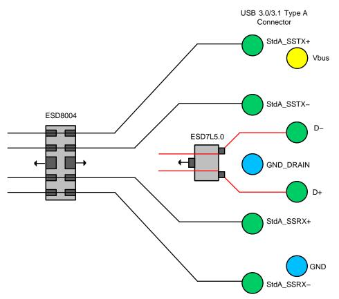
Figure 14. USB 3.0/3.1 Layout Diagram
