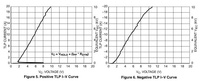
NOTE: TLP parameter: Z<sub>0</sub> = 50 Ω, t<sub>p</sub> = 100 ns, t<sub>r</sub> = 300 ps, averaging window: t<sub>1</sub> = 30 ns to t<sub>2</sub> = 60 ns. V<sub>IEC</sub> is the equivalent voltage stress level calculated at the secondary peak of the IEC 61000–4–2 waveform at t = 30 ns with 2 A/kV. See TLP description below for more information.
