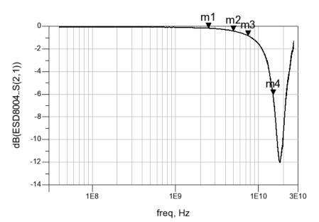
Figure 13. ESD8004 Insertion Loss
