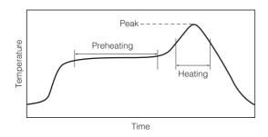
For soldering (Example : Sn/Pb)
