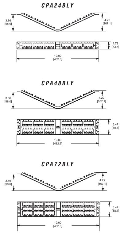
Dimensions are in inches [Dimensions in brackets are metric]
