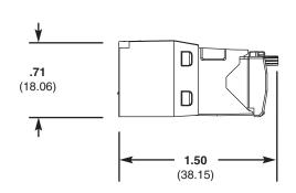
Dimensions are in inches (Dimensions in parenthesis are metric)
