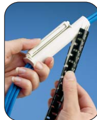
Slide Pan-Wrap™ Split Harness Wrap onto end of tool until approximately 3" of it covers the bundle.
