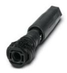
Photovoltaic connector, Range of articles: PV-C4M-S, Connector, color: black, min. conductor cross section: 2.5 mm², max. conductor cross section: 6 mm², rated current: 20 A, Connection method: Spring-cage, Type of contact: Pin
