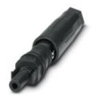
Photovoltaic connector, Range of articles: PV-C4F-S, Connector, color: black, min. conductor cross section: 2.5 mm², max. conductor cross section: 6 mm², rated current: 20 A, Connection method: Spring-cage, Type of contact: Socket
