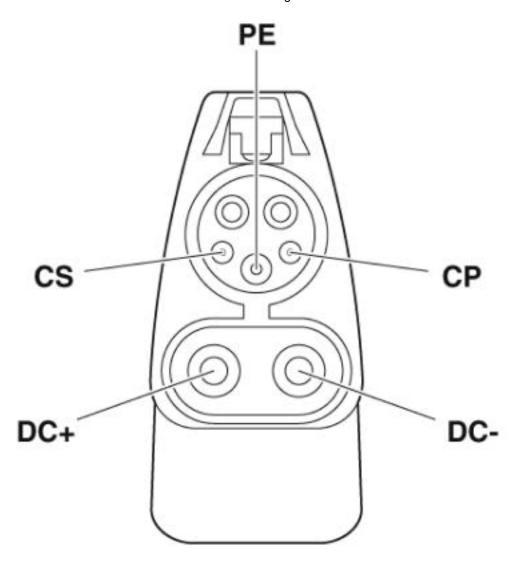
Pin assignment of the Vehicle Connector
