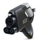
, DC charging cable with vehicle connector, open cable end, CCS type 1, Combined Charging System, SAE J1772, IEC 62196-3, 60 A / 600 V (DC), cable: 4 m, black, straight
