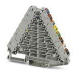
Marshalling panel, Nom. voltage: 250 V, Nominal current: 8 A, Cross section: 0.14 mm² - 2.5 mm², AWG: 14 - 26, Connection type: Push-in connection, Width: 8.3 mm, Length: 100 mm, Color: gray, Assembly: NS 35/7,5, NS 35/15
