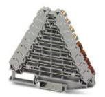
Marshalling panel, Nom. voltage: 250 V, Nominal current: 8 A, Cross section: 0.14 mm² - 2.5 mm², AWG: 14 - 26, Connection type: Push-in connection, Width: 8.3 mm, Length: 100 mm, Color: gray, Assembly: NS 35/7,5, NS 35/15
