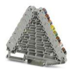
Marshalling panel, Nom. voltage: 250 V, Nominal current: 8 A, Cross section: 0.14 mm<sup>2</sup> - 2.5 mm<sup>2</sup>, AWG: 14 - 26, Connection type: Push-in connection, Width: 8.3 mm, Length: 100 mm, Color: gray, Assembly: NS 35/7,5, NS 35/15
