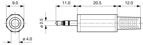
Cable diameter max. 4.0 mm
