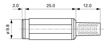
Cable diameter max. 4.0 mm
