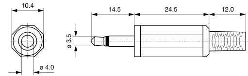
Cable diameter max. 4.0 mm
