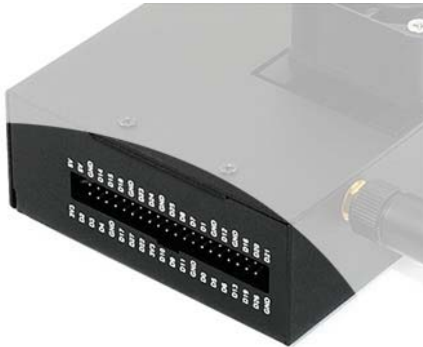
Easy access to the extension header, with clear label
