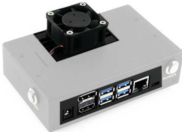
Opening for onboard connectors and cooling fan
