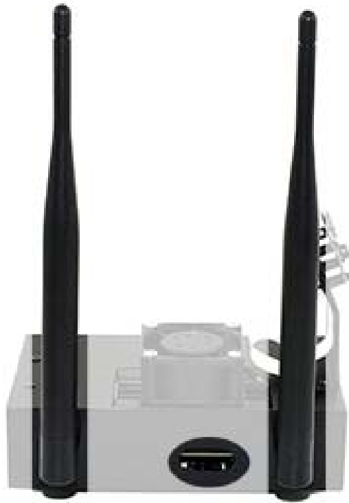
Dual antenna connectors + SD card slot
