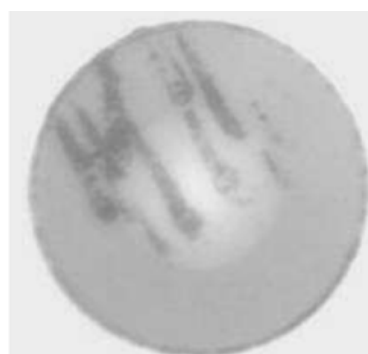
Contaminated or scratched termini endface
