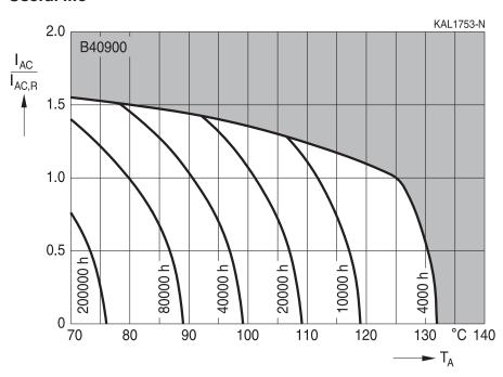
Depending on ambient temperature T<sub>A</sub> under ripple current operating condition at V<sub>B</sub> - refer to chapter "General technical information, 5 Useful life" on how to interpret useful life.
