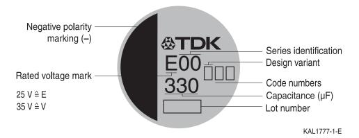
The standard coated aluminum case only serves to protect the capacitor from direct contact, but does not offer any functional insulation. Thus, this protective material must be considered as electrically non-insulating. Capacitors with such standard protective material must not be used in circuits that require electrical insulation.
