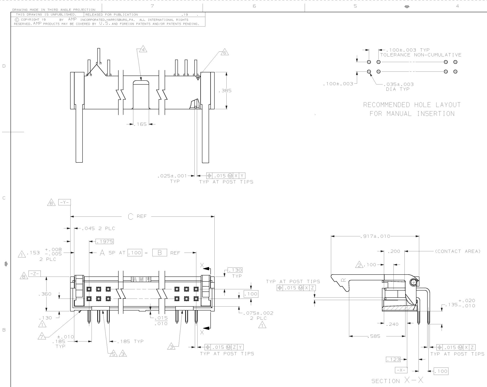
1THE NOTED DIMENSIONS APPLY AT THE INTERSECTION OF THE POST AND HOUSING  $\Delta$ POINT OF MEASUREMENT FOR PLATING THICKNESS  $\underline{\mathbb{A}}$ DOUBLE BAR POLARIZATION CENTER POLARIZATION SLOT FOR 10 POSN ASSEMBLY, SLOT OMITTED WHERE INDICATED  $\triangle$ NUMBER 1 POSITION INDICATOR.  $\triangle$ OPTIONAL AMP IDENTIFICATION NUMBER (DATE CODE). LOCATION APPROXIMATELY WHERE SHOWN.
