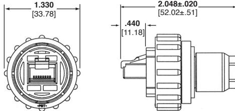
Receptacle Kit, Pass-through RJ45/RJ45 – Part No. 1776186-1
