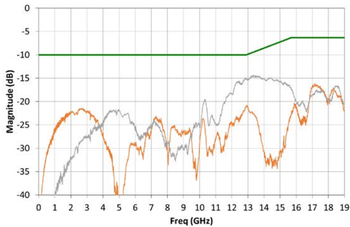
Return Loss (SDD11) of 4m 28AWG SFP28
