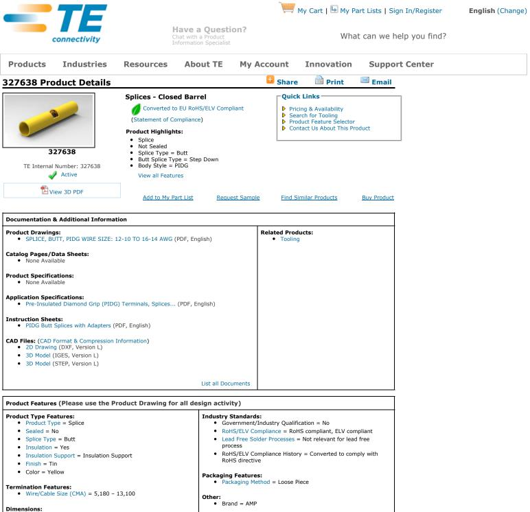
Insulation Diameter (mm [in]) = 5.59/4.32 [.220/.170] Max.
