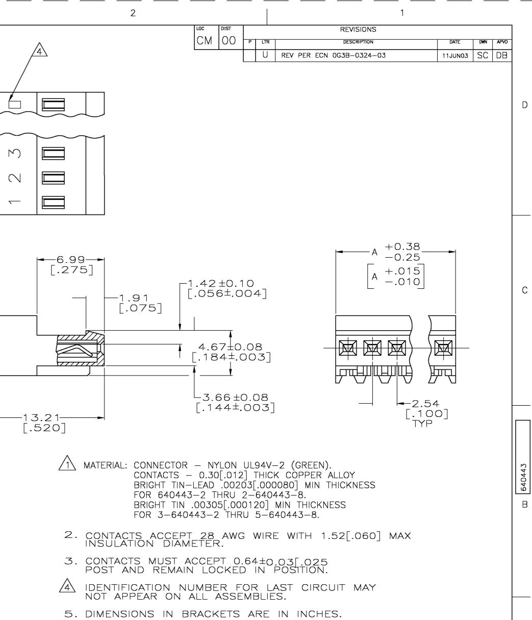
6. HOUSING FEATURES ARE: CLOSED END WITH LOCKING RAMP.
