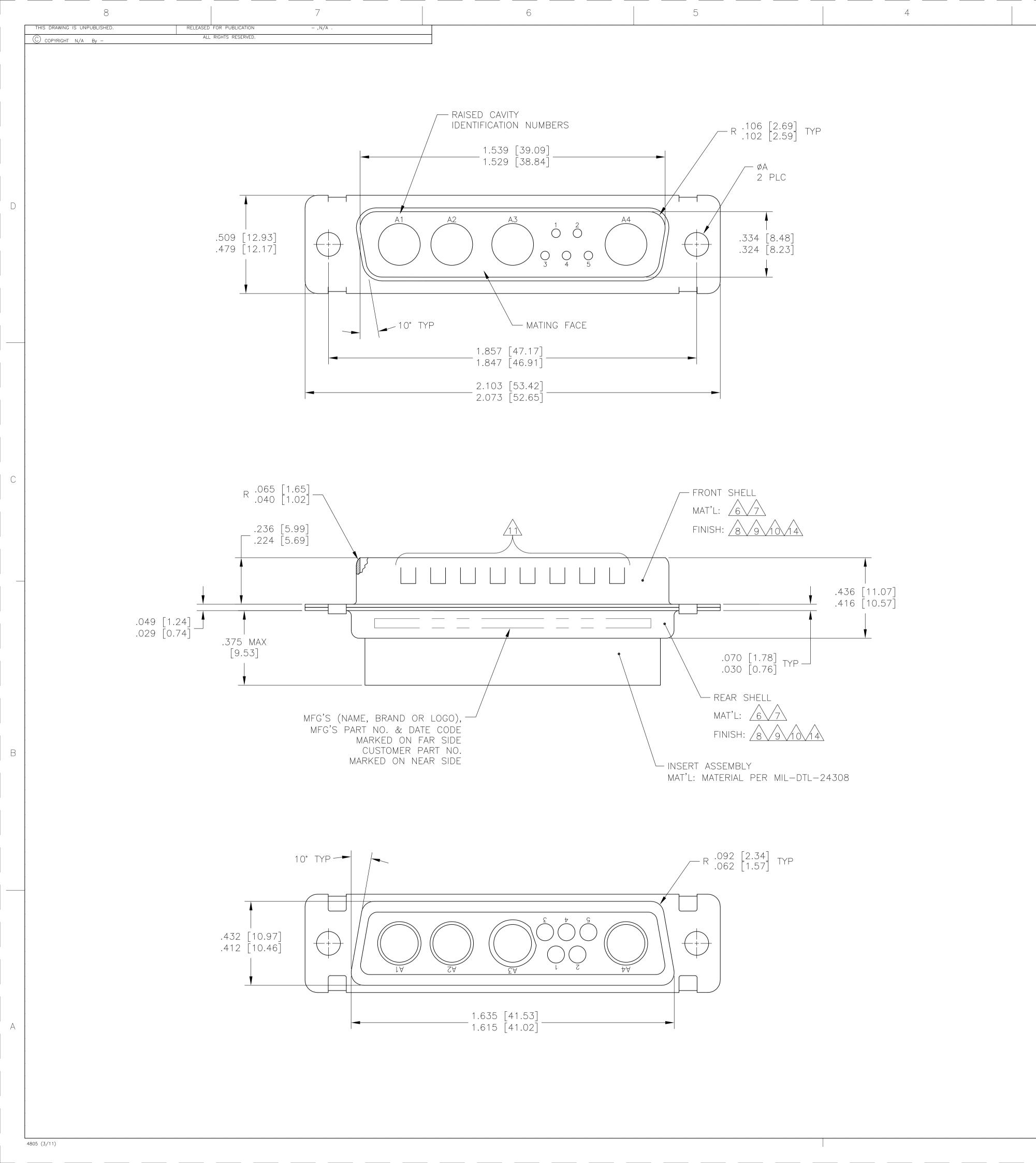
1. THIS CONNECTOR ASSEMBLY IS SUPPLIED WITH SIZE 20 METAL CONTACT RETENTION CLIPS INSTALLED IN THE INSERT ASSEMBLY.
