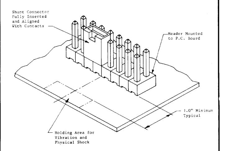
Holding Area for Vibration and Physical Shock Figure 6
