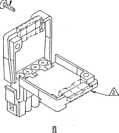
r-(2 REQ'D) #6 X .375 LG. TYPE"B" PAN HEAD SHEET METAL SCREW
