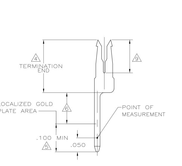
1CONTACTS DESIGNED FO Solid Wire. 2AMP TRADEMARK LOCA  $\overline{3}$ STANDOFFS: POSN 8 POSN 14-A PLATED WITH .000100 OVER .000050 NICKE  $\sqrt{5}$ PLATED WITH .000030  $\bigcirc 6 \bigcirc$ GOLD FLASH OVER .00005  $\triangle$ HEIGHT AFTER TERMI A INDICATES NO 1 POS  $\underline{\land}$ PLATED WITH .000005 .000050 MIN NICKEL.  $\overline{10}$ MOLDED PARTS: 94V—0 RA Contacts: phos bronze.
