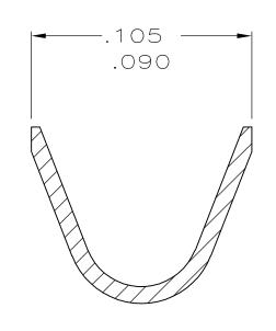
SECTION B-B INSULATION RANGE .025-.060 SCALE 20:1
