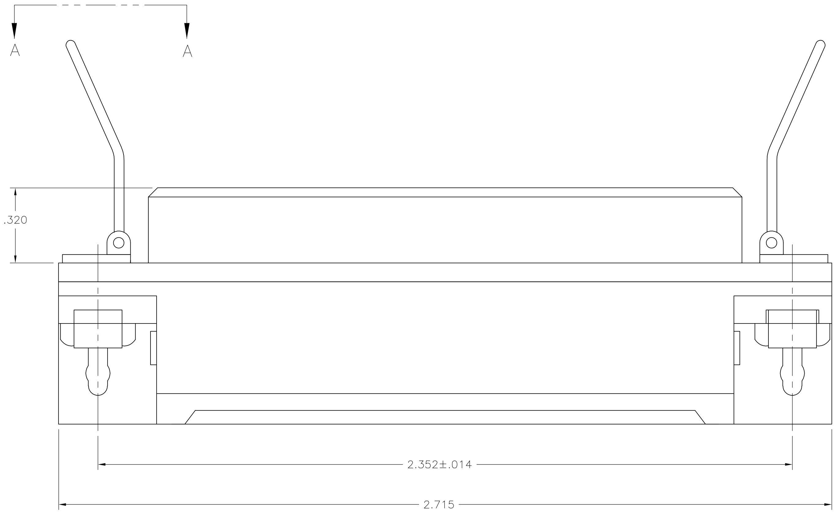
SUGGESTED PRINTED CIRCUIT BOARD MOUNTING DIMENSIONS
