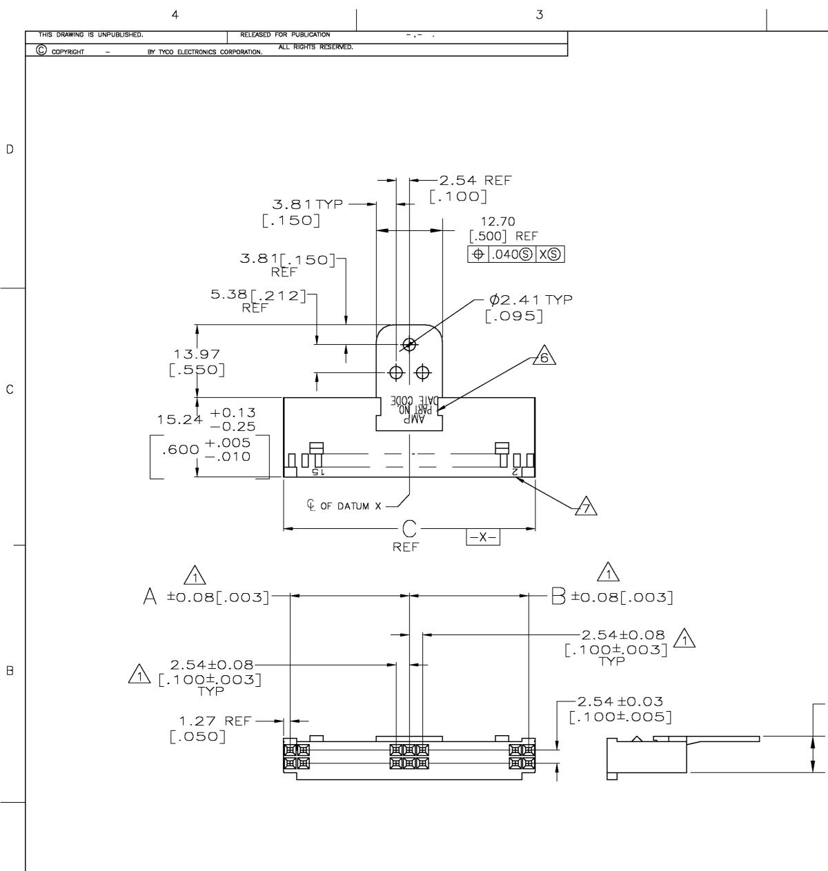
CAVITY LOCATION DIMENSIONS INCREASE IN INCREMENTS OF 2.54[.100], TOLERANCE NON-CUMULATIVE.
