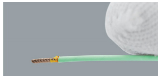
STEP 2: Strip the insulation* 5 mm maximum.
