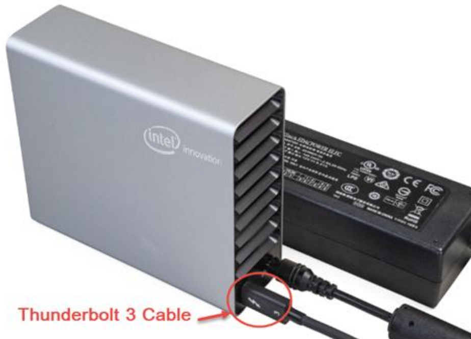
Figure 2-3 Plug the Thunderbolt 3 cable to the FLIK
