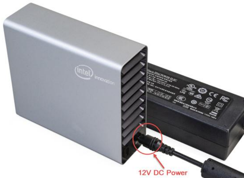
Figure 1-4 Plug the DC 12V power to the FLIK
