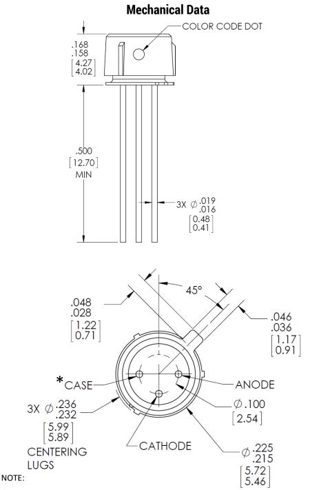
Case is electrically isolated from cathode and anode.
