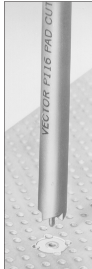
Shows pad removal & pad cutter P116C
