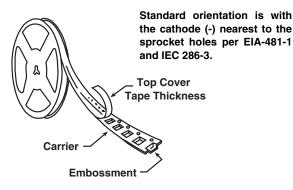
**Tape and Reel Specifications:** All case codes are available on plastic embossed tape per EIA-481-1. Tape reeling per IEC 286-3 is also available. Standard reel diameter is 13" [330 mm]. 7" [178 mm] reels are available.
